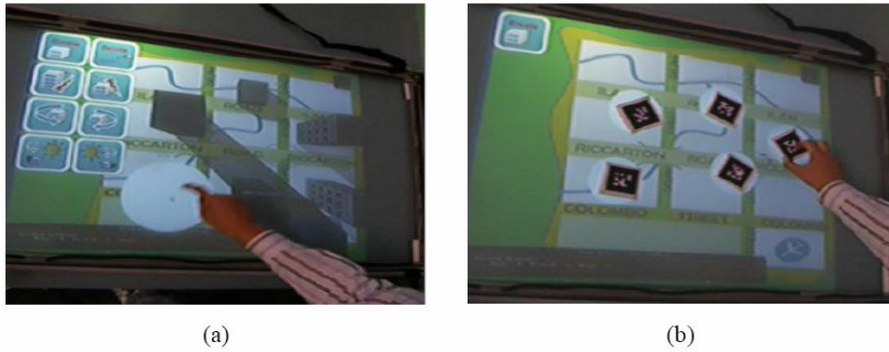
Fig. 6. The tabletop interface (a) tabletop interface recognizing hand gesture (the white circle is a clicked position) (b) physical objects on the table
